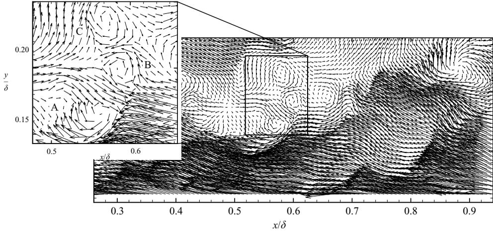
FIGURE 7. Example of a prograde hairpin vortex head (labelled A) oriented at approximately  $255^\circ$  relative to a neighbouring retrograde vortex (labelled B), as visualized by Galilean decomposition of an instantaneous velocity realization with  $U_c = 0.79U_\infty$ .
