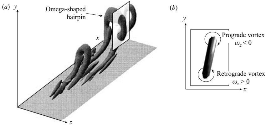
FIGURE 6. (a) Three-dimensional visualization of a hairpin vortex packet, adapted from Zhou *et al.* (1999), illustrating the existence of omega-shaped hairpin structures. (b) Spatial signature revealed if the structure in (a) were sliced through one of its shoulders by a streamwise–wall-normal measurement plane.
