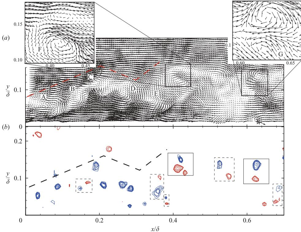
FIGURE 1. (a) Galilean-decomposed velocity field in the streamwise–wall-normal plane at  $Re_\tau = 2350$  with  $U_c = 0.81U_\infty$ . (b) Retrograde (red) and prograde (blue)  $\Lambda_{ci}$  calculated from the velocity field in (a). The dashed line highlights the tent-like interface of the visualized packet.
