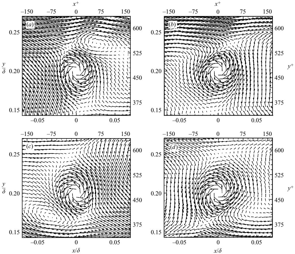
FIGURE 4. Conditionally averaged velocity fields given a retrograde vortex at  $y = 0.2\delta$  for which its closest prograde vortex is oriented in quadrants (a) one, (b) two, (c) three and (d) four relative to the retrograde core.
