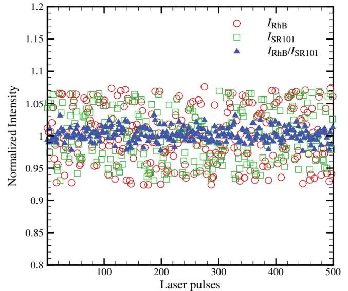
**Figure 4.** Variation of the fluorescence emission from the two dyes as a function of number of laser pulses used for illumination of the dyes. The dye solution is continuously flowing to avoid photobleaching effects.
