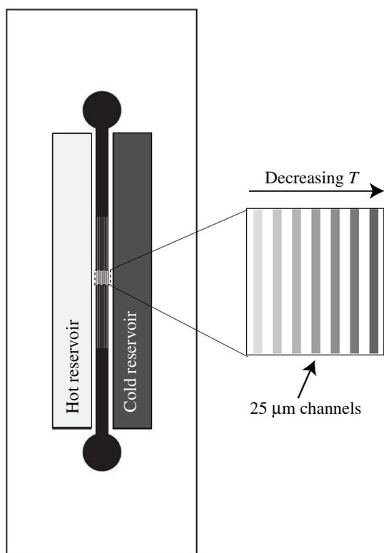
**Figure 9.** Schematic of the device utilized to obtain a one-dimensional, steady-state temperature gradient at the microscale.
