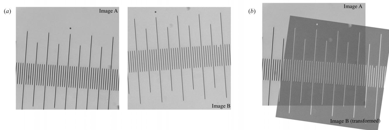
**Figure 2.** (a) Images of a target acquired simultaneously with cameras  $\alpha$  and  $\beta$ , respectively, used to register the cameras relative to one-another. (b) Result of applying a transformation to image B via a geometric mapping function.
