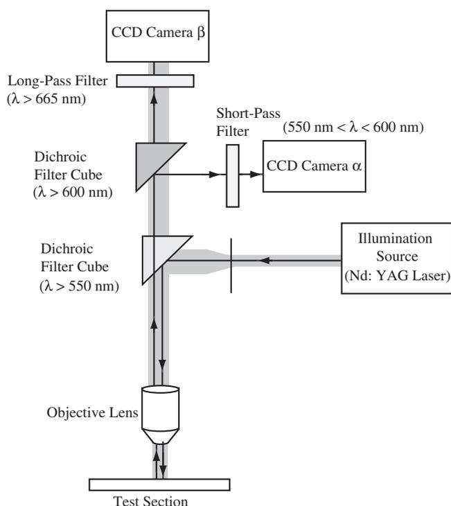
**Figure 1.** Schematic of the experimental arrangement for two-color LIF at the microscale.
