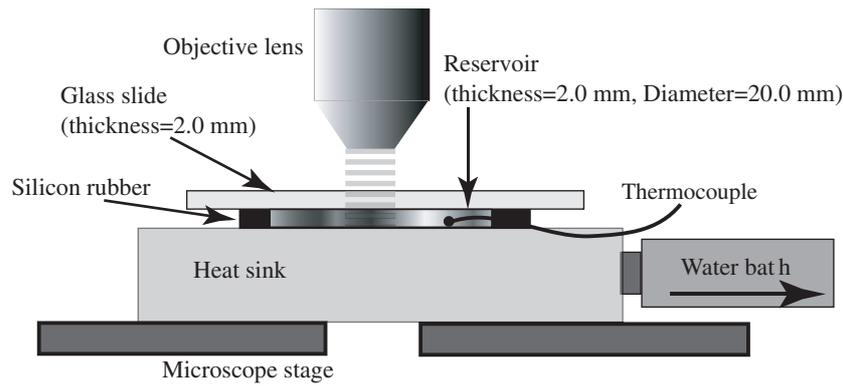
Figure 5. Schematic of the microfluidic device used to calibrate the temperature dependence of RhB and SR101.
