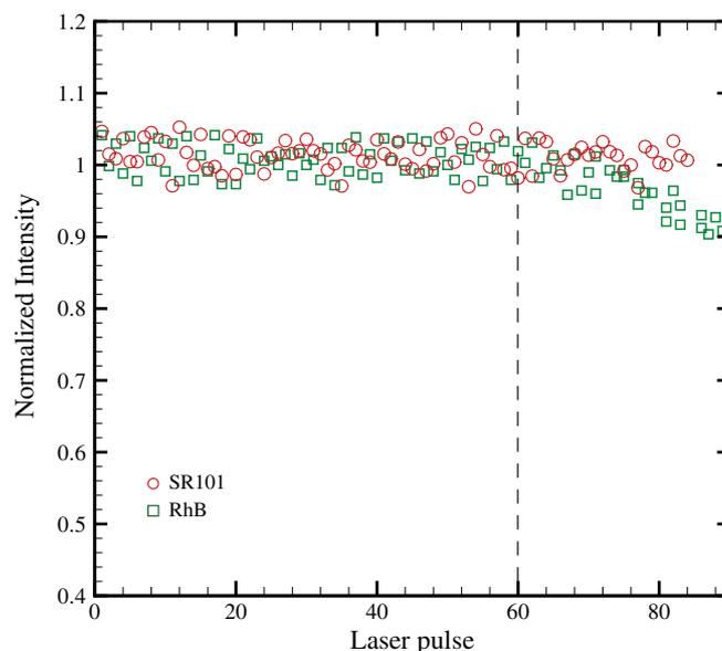
**Figure 8.** Variation of the emission intensity of RhB and SR101 as a function of number of laser pulses used for illumination of the dyes illustrating the onset of photobleaching in the case of RhB. The measured intensities are normalized by the mean intensity at 20 °C ( $I_{20}$ ).
