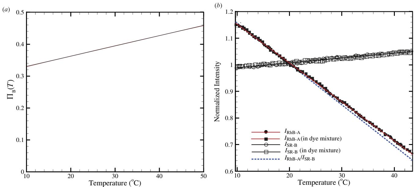
Figure 6. (a) Variation of  $\Pi_B$ , the ratio of the emission from SR101 dissolved in ethanol, imaged by cameras  $\alpha$  and  $\beta$ , respectively, as a function of temperature. (b) Temperature dependence of the fluorescence emission of SR101 and RhB dissolved in ethanol. The measured intensities are normalized by the intensity at 20°C ( $I_{20}$ ).
