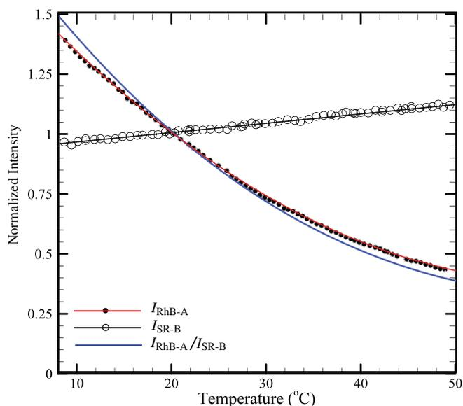
**Figure 7.** Temperature dependence of the fluorescence emission of SR101 and RhB dissolved in water. The measured intensities are normalized by the intensity at 20 °C ( $I_{20}$ ).
