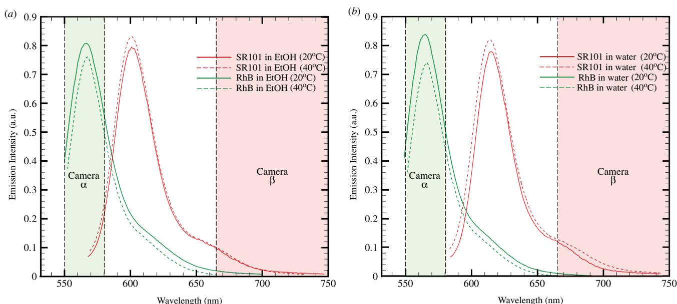
**Figure 3.** Emission spectra of RhB and SR101 dissolved in (a) ethanol and (b) water at 20 °C and 40 °C when excited at 532 nm. The shaded regions demarcate the wavelengths that are imaged by cameras  $\alpha$  and  $\beta$  in the experimental arrangement presented in figure 1.
